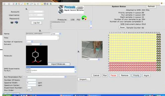
Log in samples quickly and monitor analytical progress from any web browser. Or import sample lists directly from your HPLC or other instruments. Support for 96 or 384 well microplates and your choice of low-volume vials. Supports up to three solvents.
